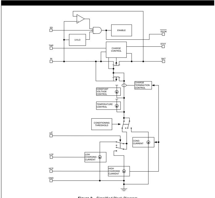
Figure 2 - Simplified Block Diagram
